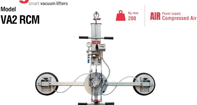
The model VA2 RCM is a **vacuum glass lifter specific for indoor use**, with two suction pads d. 310 mm, compressed air powered with lifting capacity up to 200Kg. The pads are replaceable along the arms in different positions.
