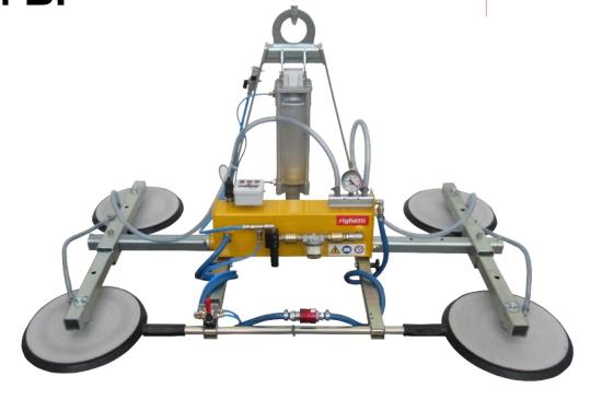
The model VA4 BP is a **vacuum glass lifter specific for indoor use**, with four suction pads d. 310 mm, compressed air powered with lifting capacity 400Kg. The pads are replaceable along the arms; and the arms are replaceable along the central beam, which is long 1500 mm.
