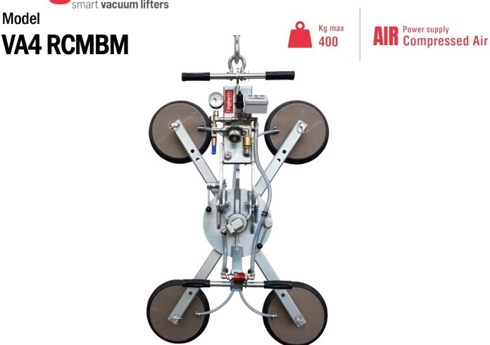
The model VA4 RCMBM is a **vacuum glass lifter specific for indoor use**, with four suction pads d. 310 mm, compressed air powered with lifting capacity 400Kg. The pads are replaceable along the arms in two different positions.
