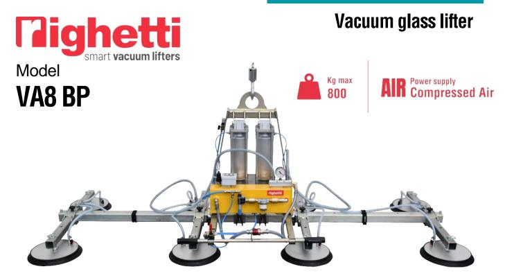
The model V84 BP is a **vacuum glass lifter specific for indoor use**, with eight suction pads d. 310 mm, compressed air powered with lifting capacity 800Kg. The pads are replaceable along the arms; and the arms are replaceable along the **central beam, which is long 2500 mm**.
