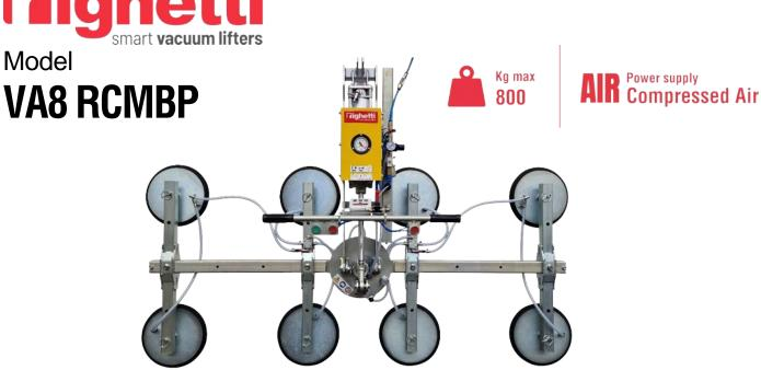
The model V84 RCMBP is a vacuum glass lifter specific for indoor use, with eight suction pads d. 310 mm, compressed air powered, with lifting capacity 800Kg. The pads are replaceable along the arms; and the arms are replaceable along the **central beam**, which is long 2500 mm, as standard.
