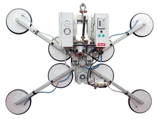
The model VB4+4 RCEBE d4 is a **modular vacuum glass lifter** with electric movements. On VB4+4 model, the four external suction pads are on removable extension arms that permit to increase the lifting capacity and the pad spread. The pad arms can be removed quickly and easily.
