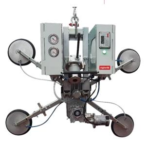
The VB4 RCEBE d4 PRO is a version of the standard VB4 vacuum glass lifter completed with four **extension arms** for bigger pad spread. Thanks to its extension arms, this lifter can reach **four different configurations**. The four suction cups can be put **in in-line position** and allow the lifter to handle long and narrow glass.
