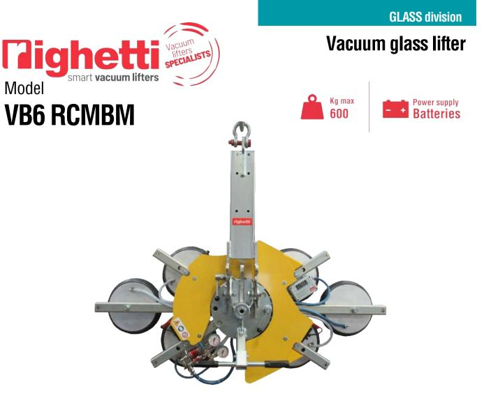
The VB6 RCMBM is a vacuum glass lifter with **manual 360° continuous rotation** and **manual tilting system** 0-90°. It has 6 round pads d. 310mm. The pad spread dimension is mm 1420 x 678.
