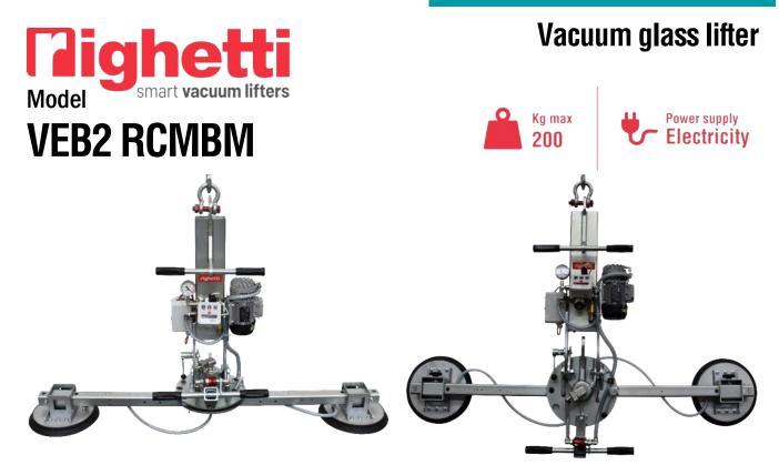
The VEB2 RCMBM model is vacuum glass lifter with two suction pads d. 310 mm, perfect to lift and handle glass sheets. VEB2 has **electric operating system**. As standard is available 400V 3 phase or 220V single phase operated system. On request other voltages.
