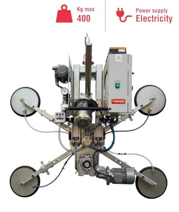
The model VEB4 RCEBE PRO is a **modular vacuum glass lifter** completed with four extension arms for bigger pad spread. Thanks to these extension arms, this lifter can reach four different configurations. The four suction cups can be put in in-line position and allow the lifter to handle long and narrow glass.
