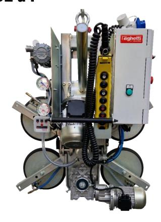
The model VEB4 RCEBE d4 is a **modular vacuum glass lifter** with electric movements and lifting capacity 600kg. The VEB4 RCEBE d4 features **powered tilt 0 – 90° and powered continue 360° rotation**. The aspiration, release, tilting and rotating commands are controlled by push button cable command (radio remote control as optional).
