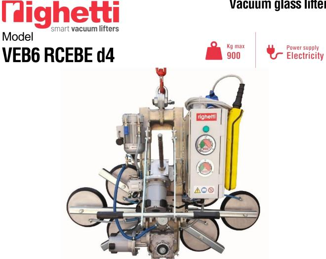
The model VEB6 RCEBE d4 is a vacuum glass lifter with electric movements and lifting capacity 900kg. The VEB6 RCEBE d4 features powered tilt 0 – 90° and powered continue 360° rotation. The aspiration, release, tilting and rotating commands are controlled by push button cable command (radio remote control as optional).
