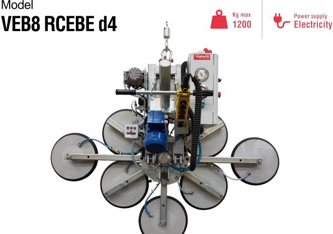
The model VEB8 RCEBE d4 is a **vacuum glass lifter** with electric movements and lifting capacity 1200kg. The VEB8 RCEBE d4 features **powered tilt 0 – 90° and powered continue 360° rotation**. The aspiration, release, tilting and rotating commands are controlled by push button cable command (radio remote control as optional).
