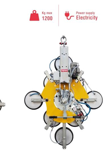
The VEB8 RCMBM d4 model is vacuum glass lifter with eight suction pads d. 390 mm, perfect to lift and handle glass sheets. VEB8 has **electric operating system**. As standard is available 400V 3 phase or 220V single phase operated system. On request other voltage.
