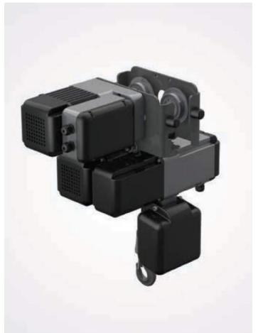
The range of the electric chain hoists is produced in 3 sizes: "VK2" - "VK3" - "VK4"; for capacity from 125 to 2.000 kg; in the FEM service groups FEM 2m (ISO M5) and FEM 3m (ISO M6); with one or two lifting speed (4 m/min - 8 m/min - 16 m/ min or 4/1 m/min - 8/2 m/min - 16/4 m/min); with standard lifting height up to 12 m.
