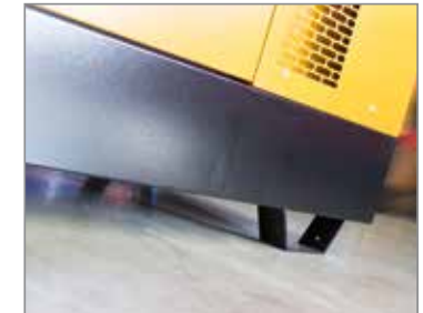
▲ Lifting points on baseframe Points de levage
